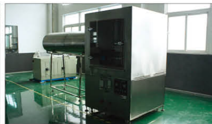
Water-proof Class Testing System
