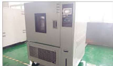
High-low Temperature Testing
